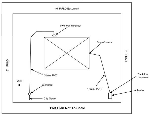
**NOTE:** All potable water openings and outlets, hose connection, shall be protected by backflow preventer. FBC – Residential P2902-3
